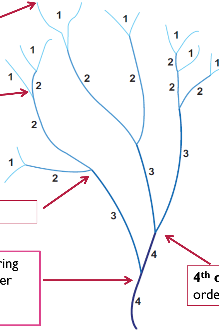
Figure 2. Stream ordering using the Strahler stream ordering system.
